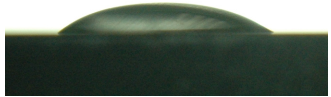
Fig. 5. Static wall contact angle measurement for water with surfactant ( \sigma = 0.042 N/m).
